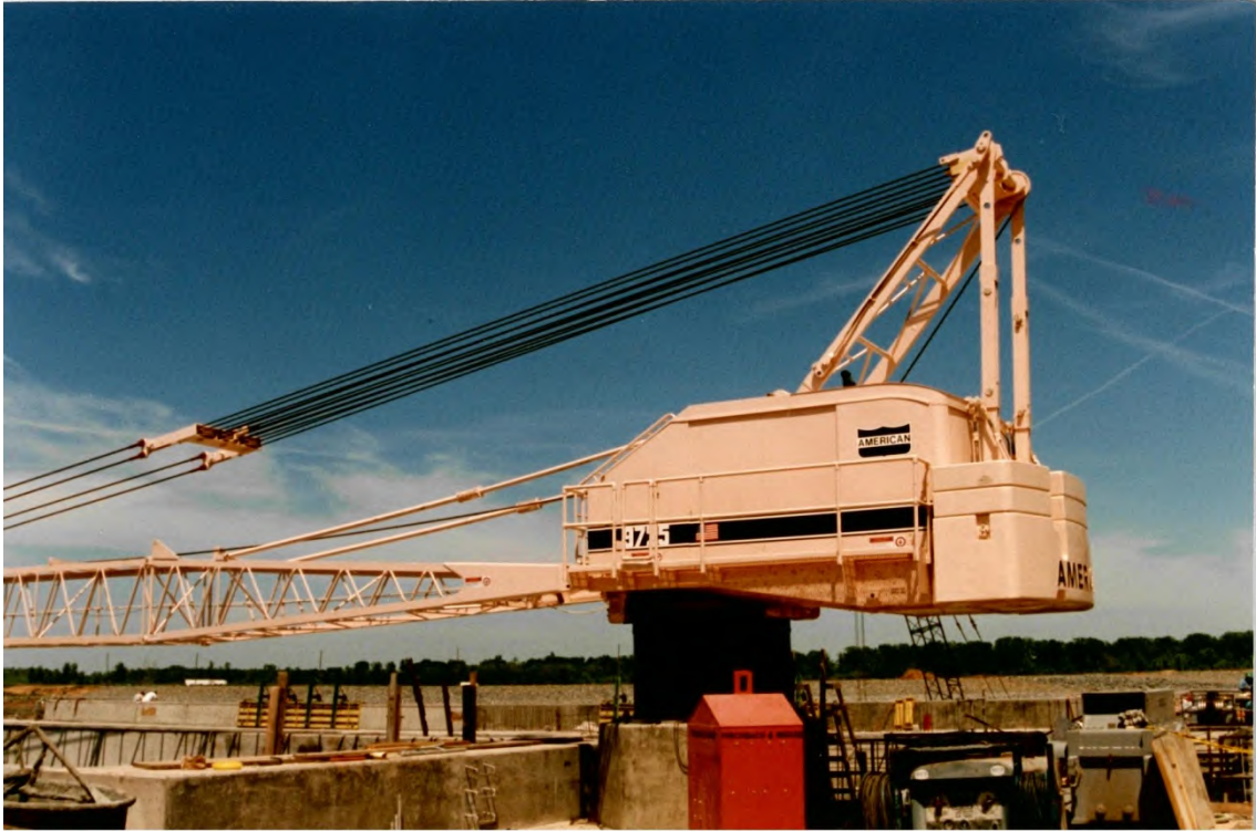
Figure 16-3. Pedestal Mounted Crane for Lifting Bulkheads.
